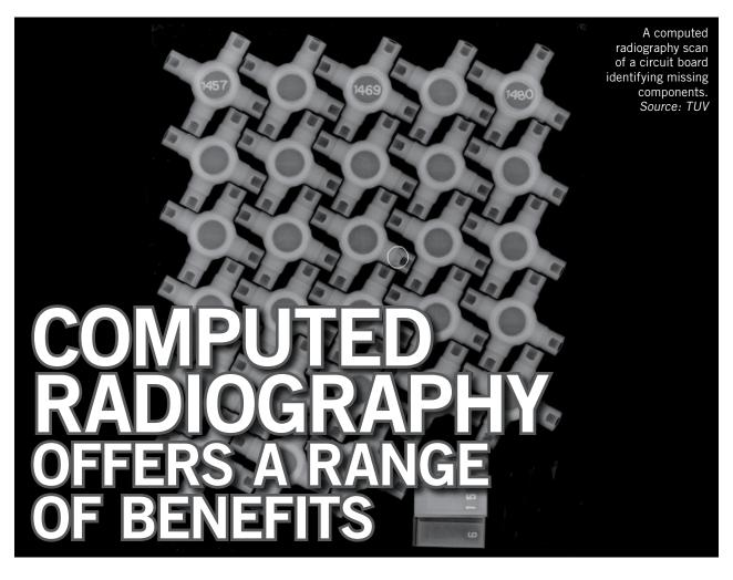
As more inspectors have turned to CR, the inspection equipment has been steadily improving, offering manufacturers faster and more precise and cost-effective NDT results than ever before.
