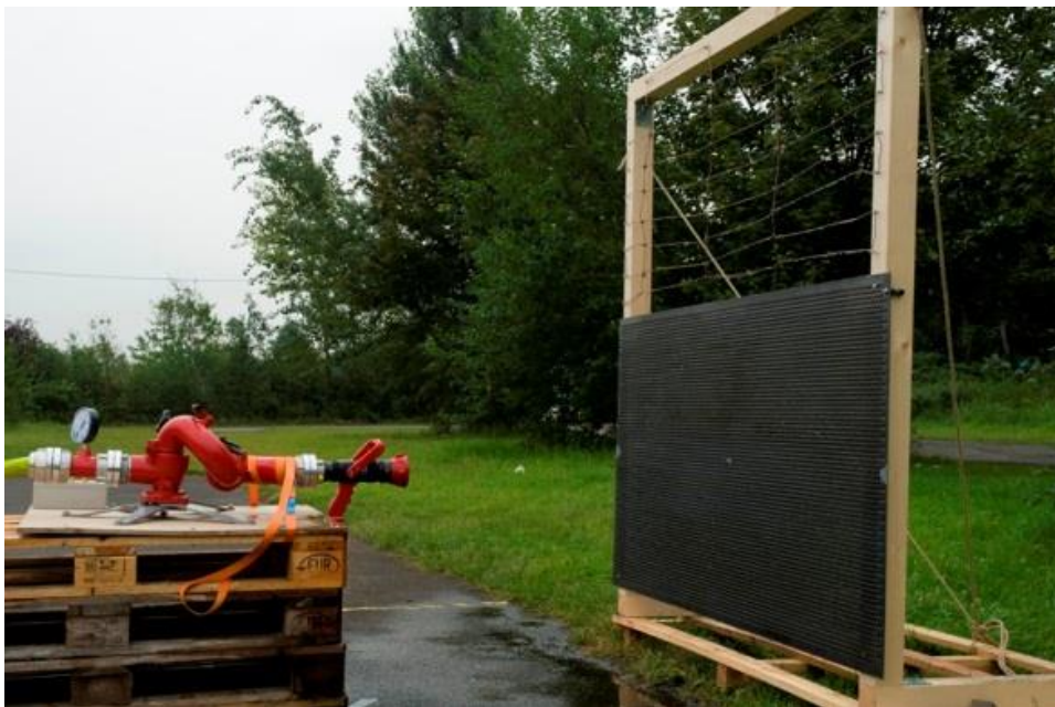
Figure 4-8: Test setup with simulated PV module (perforated plate electrode) and hollow jet nozzle at a distance of 1 meter
