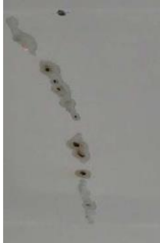
Figure 5-6: Marks along the cell fracture as the result of scorching and light flashes
