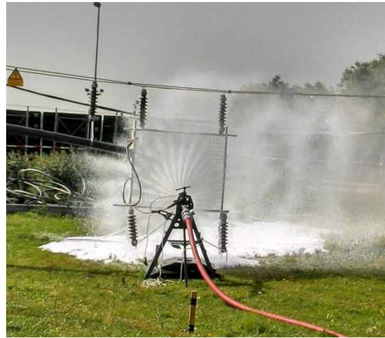
Figure 4-18: Measurement of leakage currents, extinguishing with foam under spray setting. Tests conducted on the premises of OVAG in 2014
