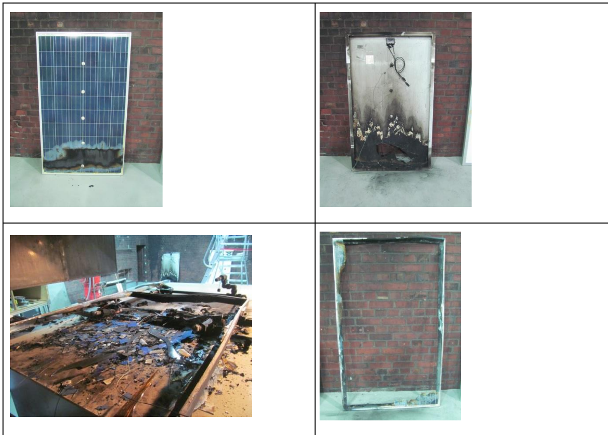
Figure 4-37: Degree of damage with c-Si and 25 kW burner output (top) and 150 kW (bottom)
