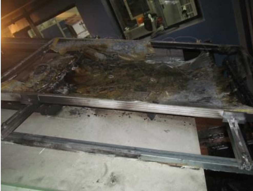
Figure 4-38: Fire residue from 2 CIGS modules: Al frame, fused glass, baked plastic residue, soot and ash
