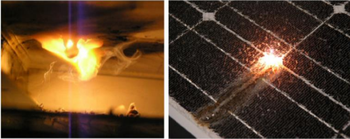
Figure 3-42: Effects of an induced electric arc through partition of the cell connectors, photos: TÜV Rheinland
