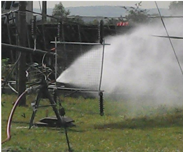
Figure 4-17: Measurement leakage currents when extinguishing live electrical installations. Tests conducted on the premises of OVAG in 2014, cooperative project of OVAG and vfdb
