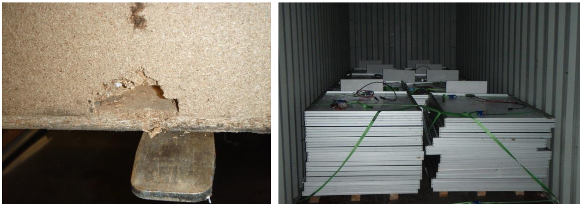
Figure 5-22: Left: incorrect handling with pressure from forklift prongs, right: improper transport of solar modules.
