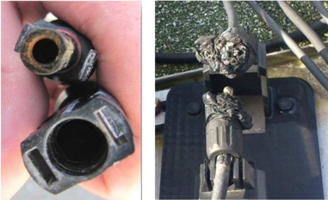
Figure 3-48: Result of pairing connectors from different manufacturers [33]
