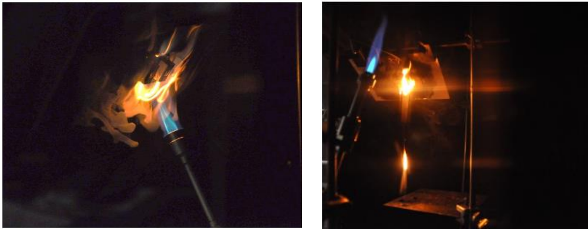
Figure 5-15: Flame impingement of lid in area of the line connections and flame impingement of the screwed cable gland of a specimen [source: TÜV Rheinland]
