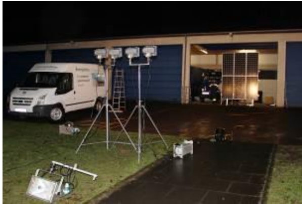
Figure 4-25: Halogen operational emitters of THW Siegburg illuminate a compact construction of six modules
