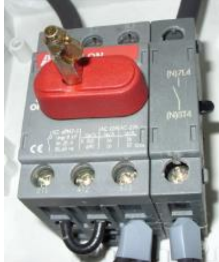
Figure 3-26: Tested DC main switch with contact rocker
