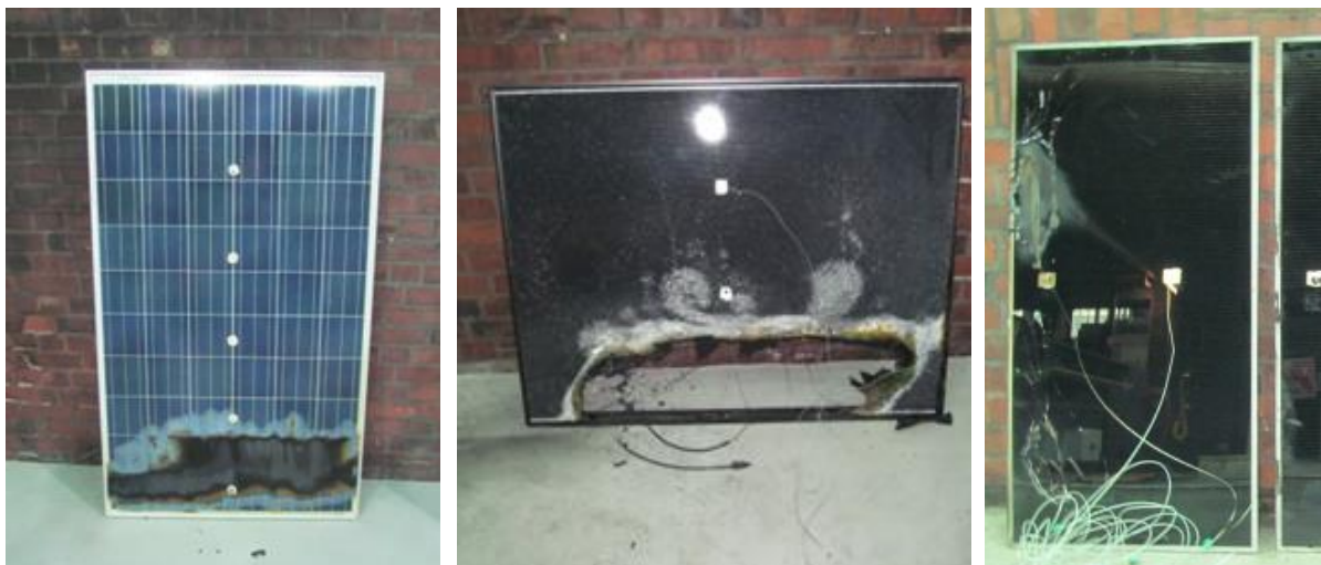
Figure 3-2: Damage from stress with 25 kW burner output, left: c-Si, center: CIS (transversely placed), right: CdTe (transversely placed)
