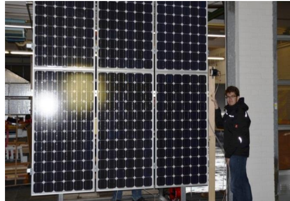
Figure 4-26: Measurement of the irradiance on the module plane produced by the emitters (above, below, on side and centered)
