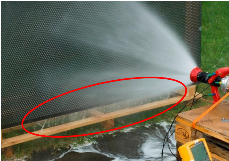
Figure 4-15: Run-off water forming conductive tracks to the wet ground – here spray jet
