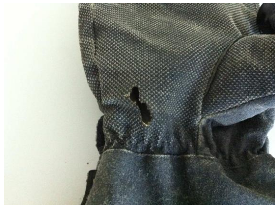
Figure 4-20: Effects of the current on the contact surfaces, burn hole from action of current
