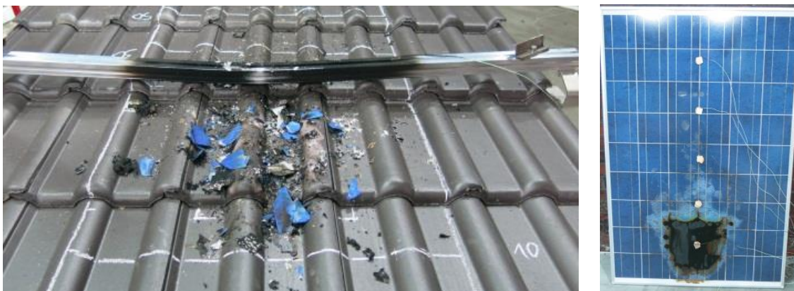
Figure 5-32: Result after test. Module was destroyed, no burn-through at the roof surface.
