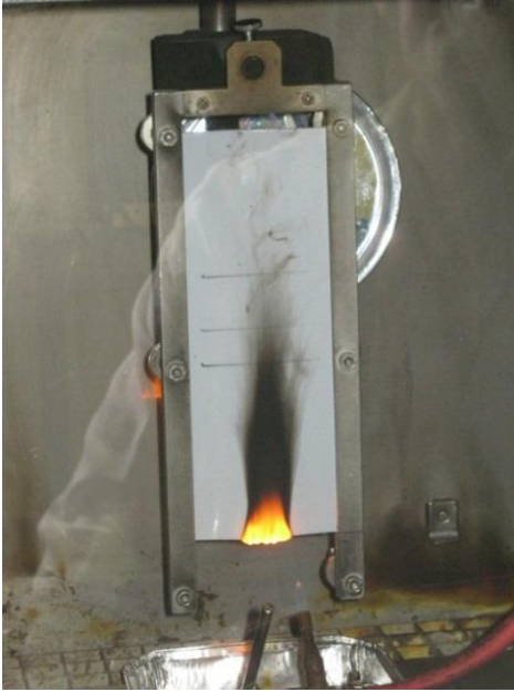
Figure 5-12: Test method for flammability as per EN 13501-1
