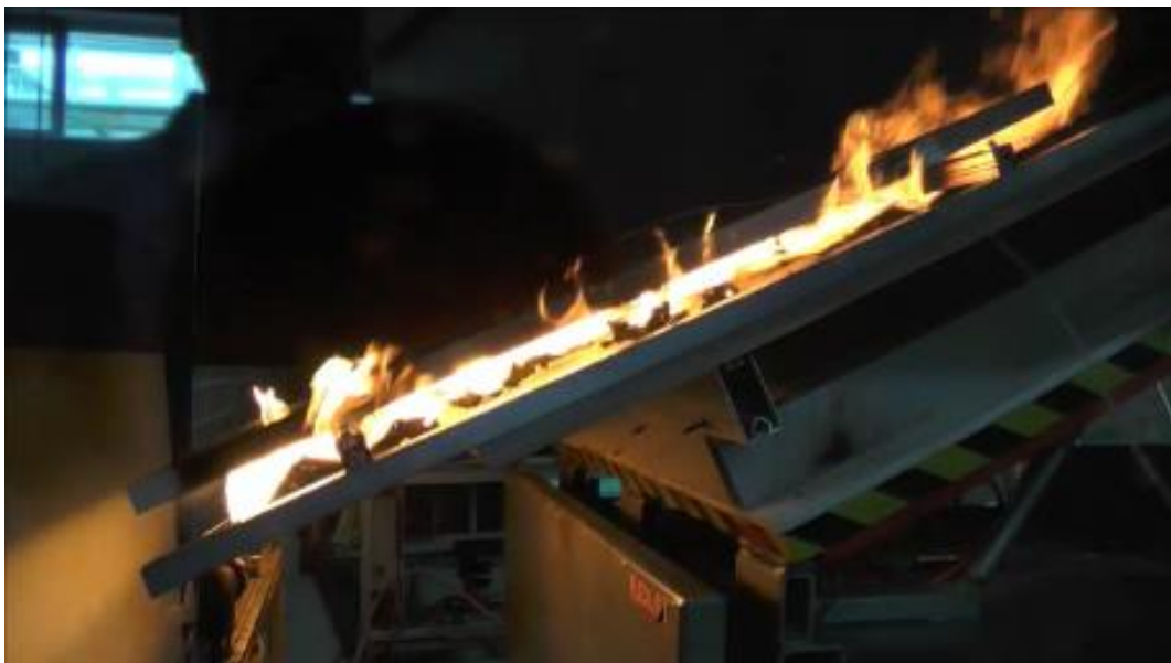
Figure 4-36: Fire test with a burner output of 25 kW (top) and 150 kW (bottom)
