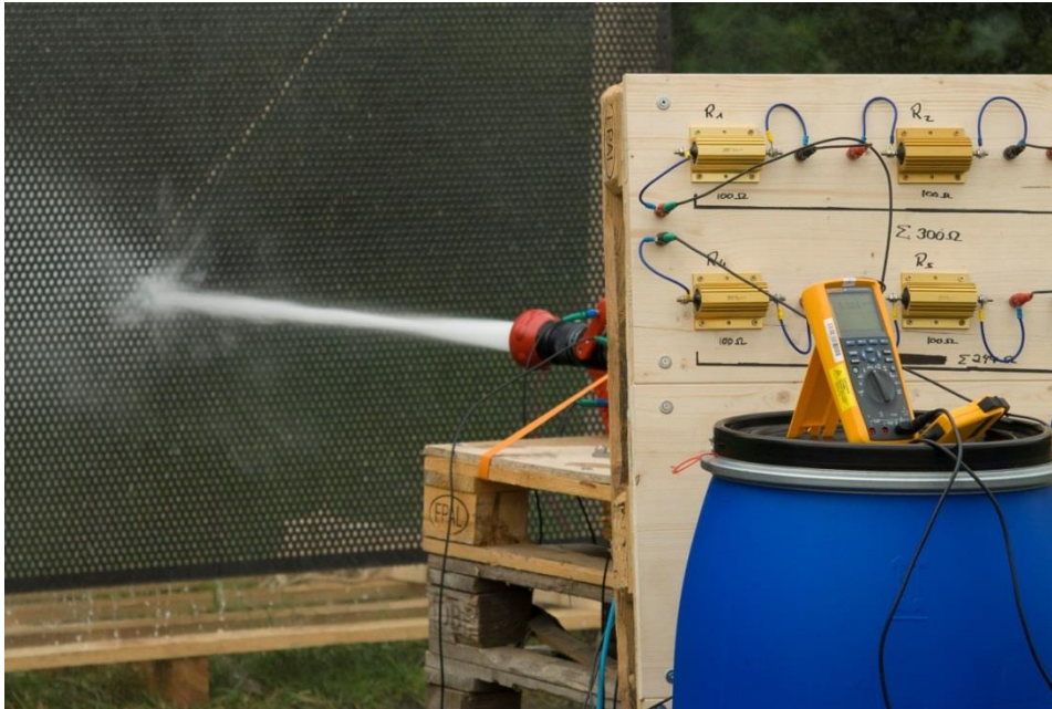
Figure 4-9: Test setup with simulated bodily resistance for measuring the leakage currents via the extinguishing stream
