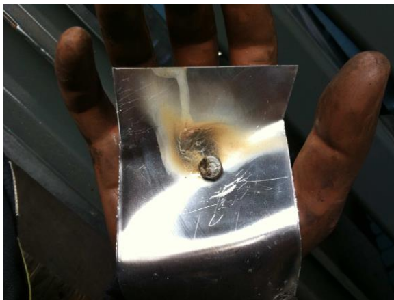
Figure 4-20: Effects of the current on the contact surfaces, burn hole from action of current
