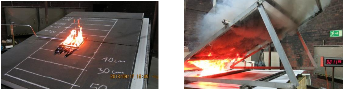
Figure 5-30: Left: elastomer bitumen sheet underlay, EPS insulating boards, bitumen vapor lock sheet with new gas burner. Right: PVC roof sealing sheet, mineral wool insulating boards, bitumen vapor lock sheet.
