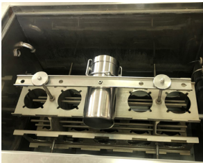
Laundering procedure in steel canister
