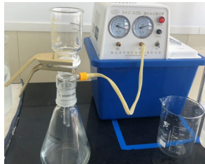
Filtration procedure first step: vacuum pump filtration
