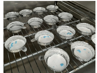
Filtration procedure second step: drying of the specimen trays
