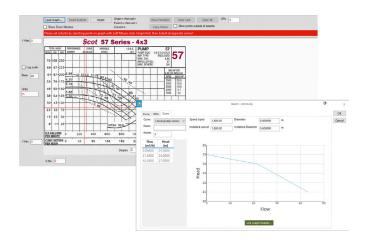
The new graph reading tool makes it easy to import data from manufacturer's pump curves in your PEL Flonet and the library function allows these curves to be saved so they can be quickly reused and shared. Build your models with a range of components and fittings. Customisable, visible alerts on the drawing warn you when flows, pressures, etc. are outside expected ranges.
