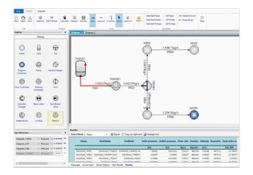
PEL Flonet calculates single phase liquid or vapour flow rates and pressure drops in piping systems. These may consist of piping loops or be 'tree-like' in form. Pumps and non-return valves can be included in the system. When supplied with the pressure at the inlets, PEL Flonet calculates the flows and internal pressures throughout the network. Alternatively, given the flows and one pressure, it will calculate the pressures at all other points.
