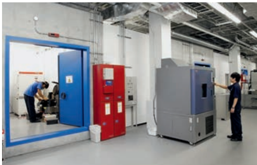
Vibrations, shock, overcharging, abnormal temperatures, moisture, or high-altitude simulations – we systematically push power storage systems to their limits at our three battery testing labs.
