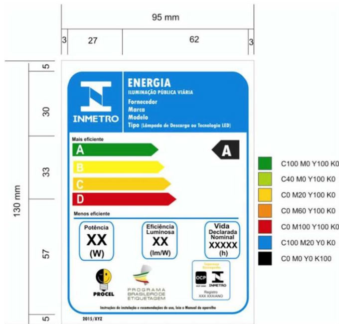
Figure 1 – ENCE - Luminaire for public lighting – LED Technology and Discharge Lamps
